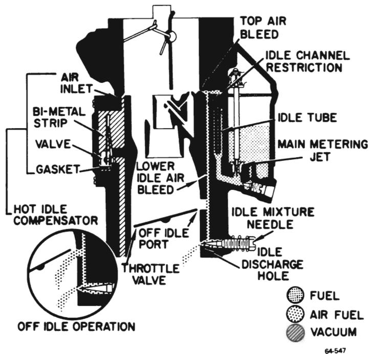
Figure 64-55 - Idle (Low Speed) System
