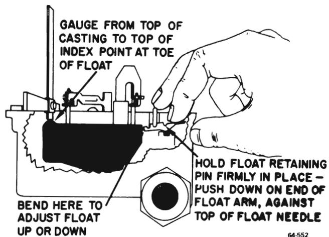
Figure 64-60 - Float Level Adjustment
