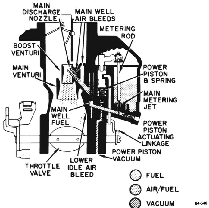
Figure 64-56 - Main Metering (High Speed) System
