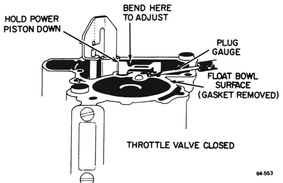
Figure 64-61 - Metering Rod Adjustment
