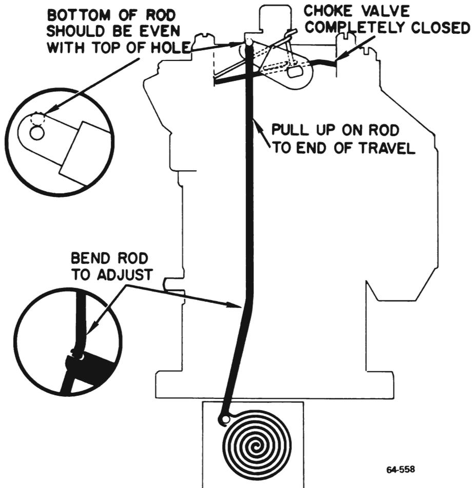
Figure 64-66 Choke Coil Rod Adjustment
