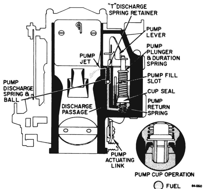
Figure 64-58 - Accelerating Pump System
