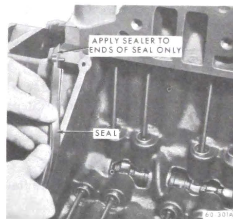
Figure 60-209 Intake Manifold Seal Installation
