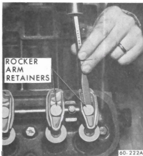
Figure 60-219 Removing Nylon Retainer
