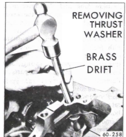
Figure 60-116--Replacing Distributor Bearing and Thrust Washer
