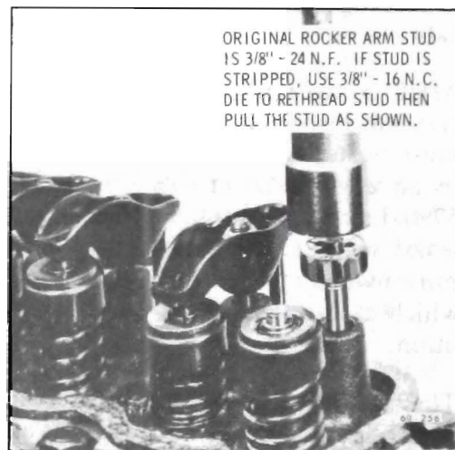
Figure 60-114 - Removing Stripped Rocker Arm Stud
