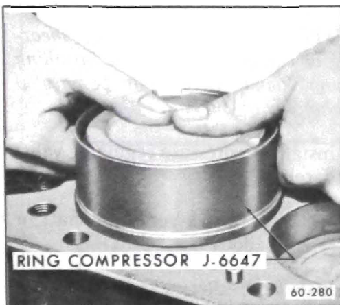
Figure 60-145 - Installing Piston with Ring Compressor
