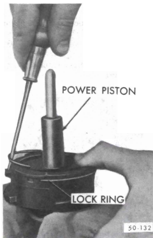
Figure 50-82 Removing Lock Ring from Power Piston
