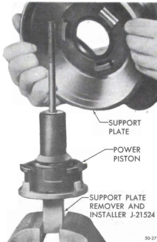
Figure 50-86 Removing Support Plate
