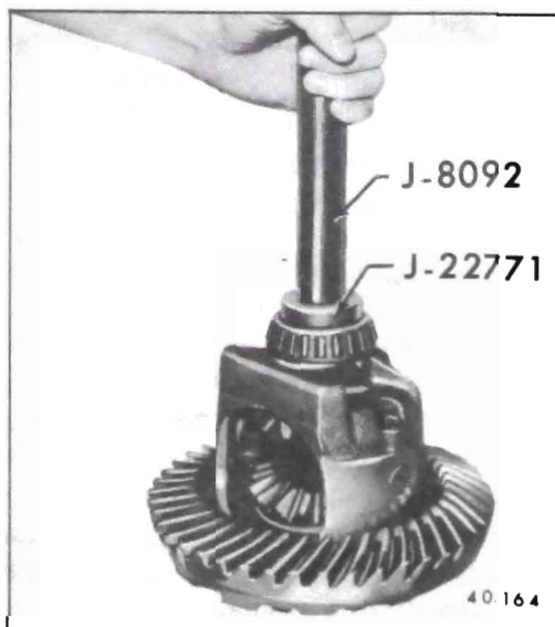
Figure 40-186 - Installing Differential Side Bearing
