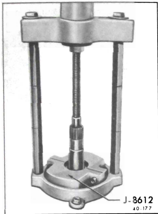
Figure 40-189 - Removing Rear Pinion Bearing
