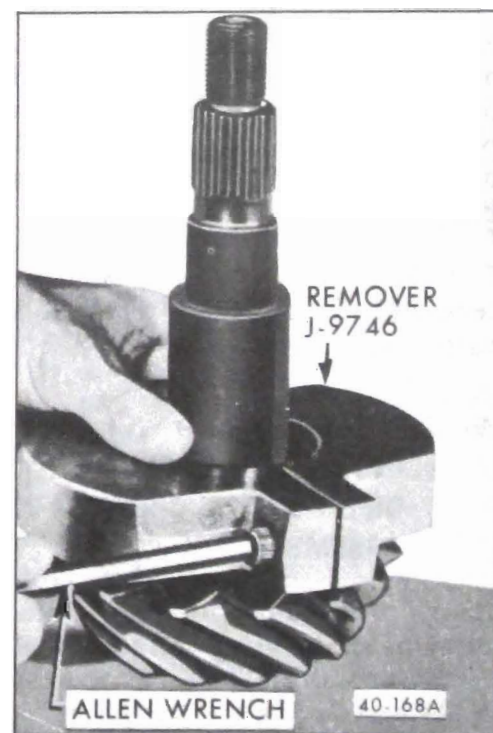
Figure 40-139 Installing Rear Pinion Bearing Remover
