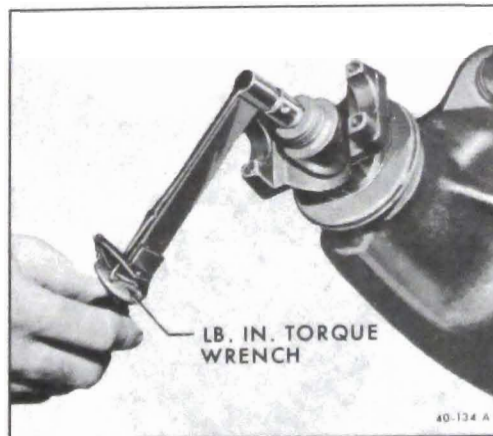
Figure 40-110 - Checking Pinion Preload
