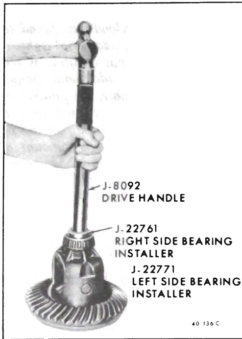
Figure 40-112 - Installing Differential Side Bearings
