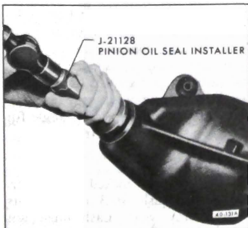
Figure 40-108 - Installing Pinion Oil Seal
