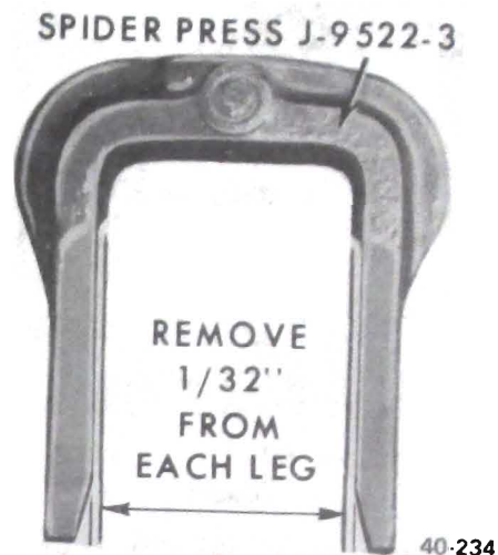
Figure 40-70 - Spider Press Leg Rework
