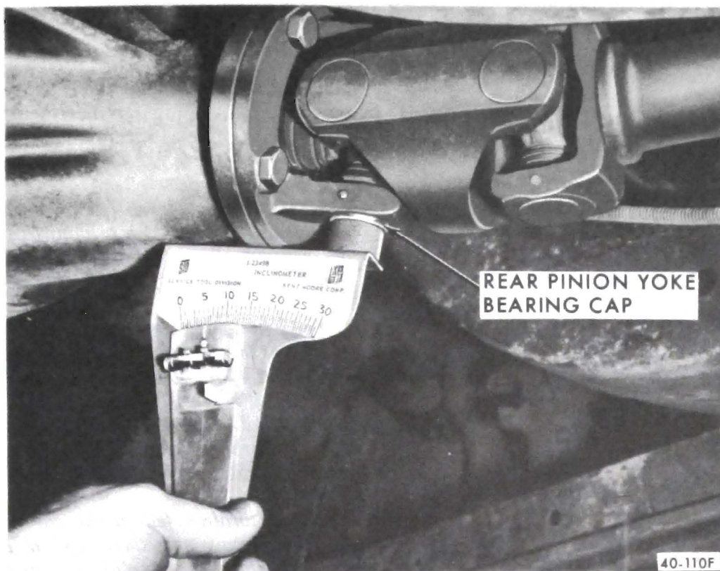
Figure 40-80B Measuring Angle at Rear of Propeller Shaft
