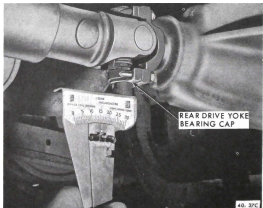
Figure 40-58 Measuring Angle at Rear of Propeller Shaft
