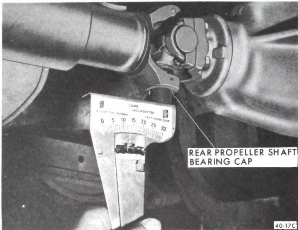
Figure 40-57 Measuring Angle at Rear of Propeller Shaft
