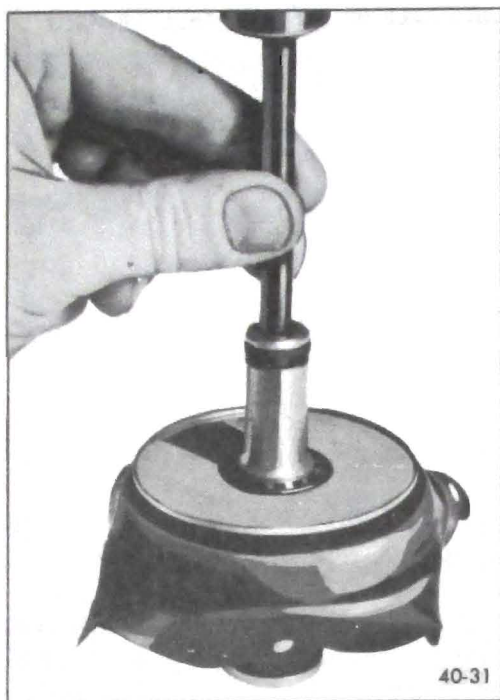
Figure 40-36 - Installing Check Valve
