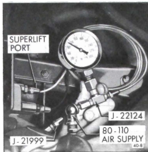
Figure 40-9 - Connect Test Gage to Superlift Outlet
