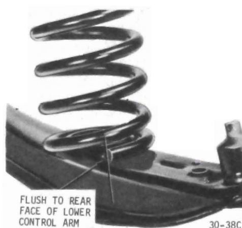
Figure 30-38 - Right and Left Front Coil Spring Position
