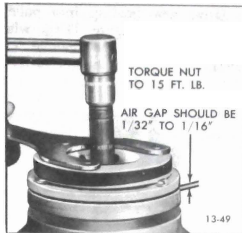
Figure 13-72 Torquing Shaft Nut
