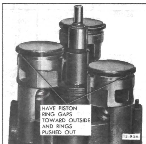
Figure 13-112 Pistons Positioned in 'Stair-Step' Arrangement
