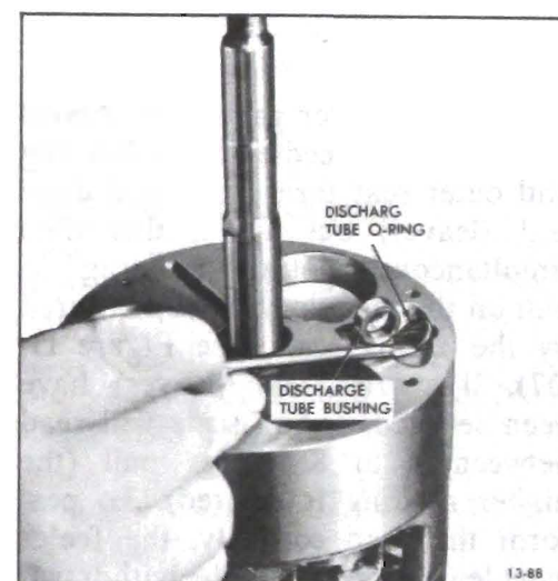
Figure 13-114 Installing Discharge Tube 'O' Ring and Bushing
