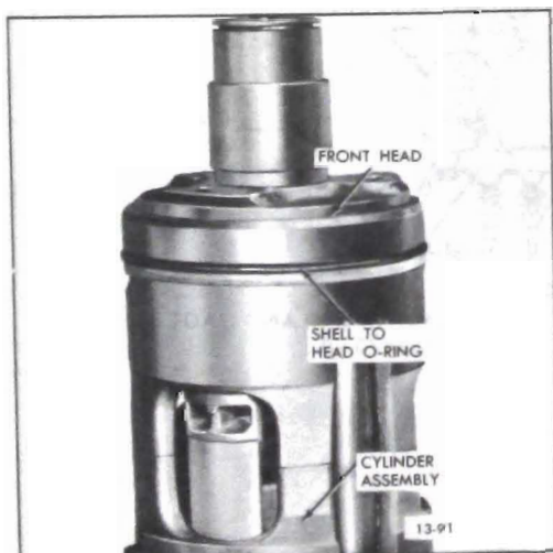
Figure 13-117 Shell to Front Head 'O' Ring Installation
