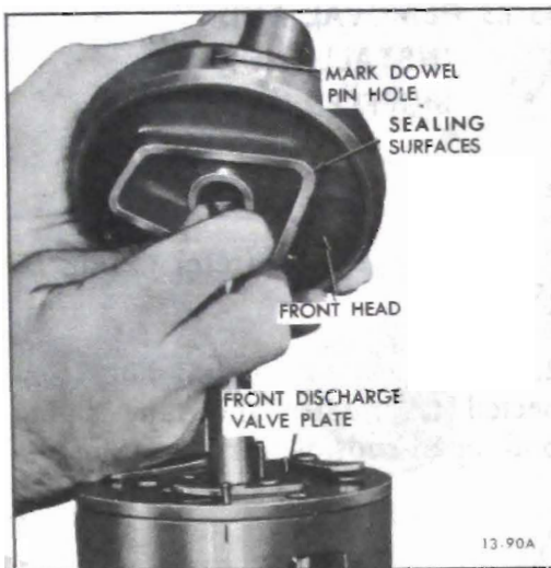
Figure 13-116 Placing Front Head on Cylinder Assembly
