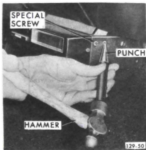
Figure 129-9 Anti-Theft Screw Loosening
