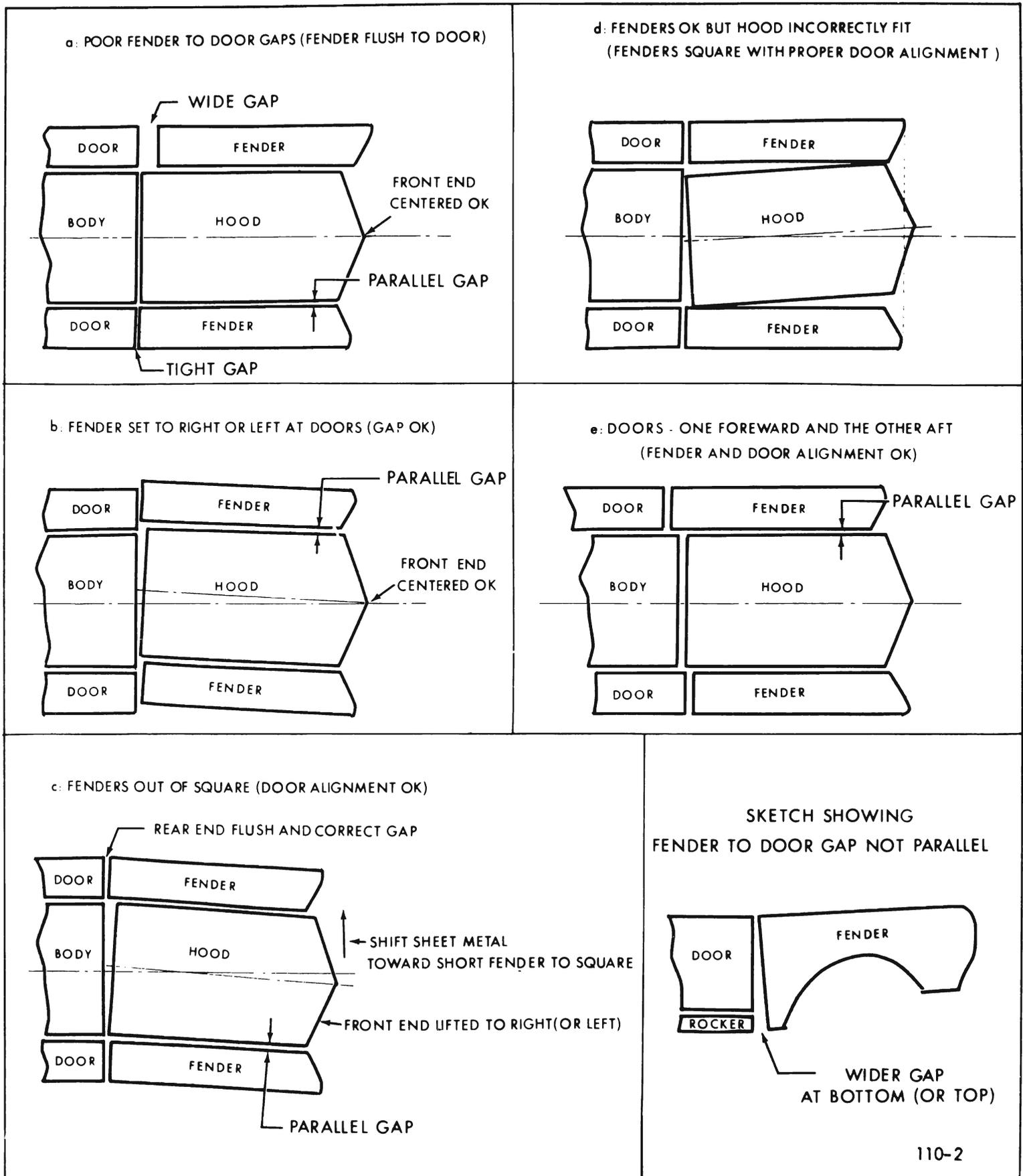
Figure 110-2—Chassis Sheet Metal Alignment
