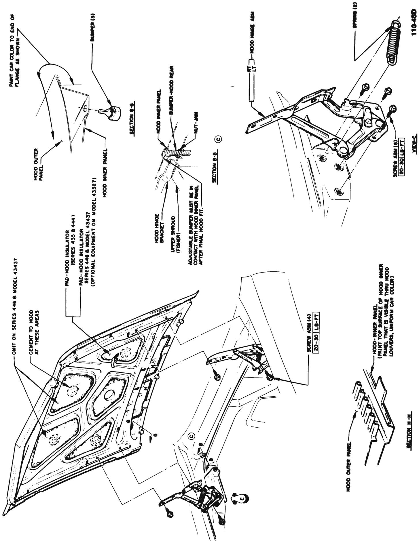
Figure 110-8 43-44000 Hood, Hood Hinge, and Hinge Spring
