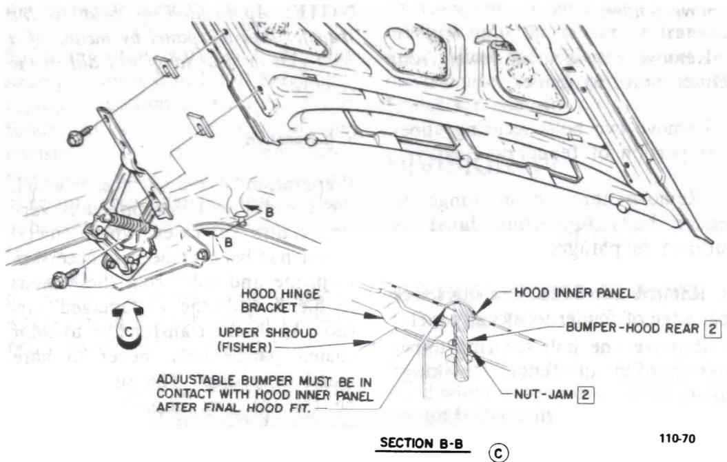
Figure 110-1 Shimming Hood to Hood Hinge
