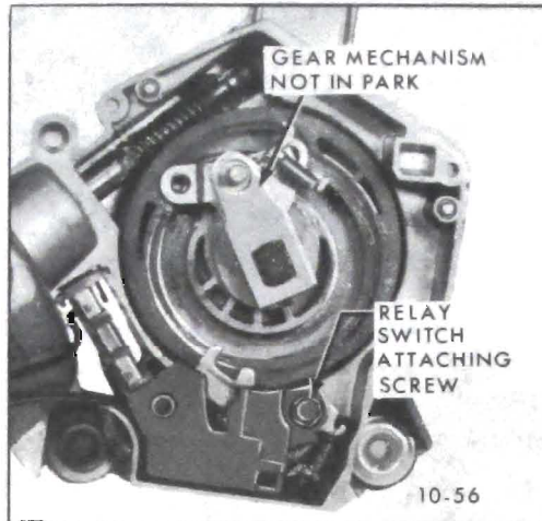
Figure 10-51 Removing Relay Switch Assembly
