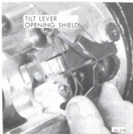
Figure 90-142 - Removing Tilt Lever Opening Shield
