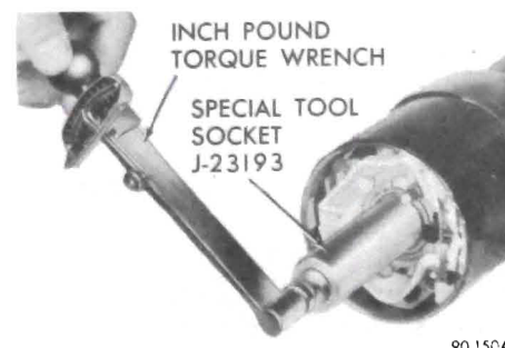
Figure 90-151 - Adjusting Steering Shaft Torque
