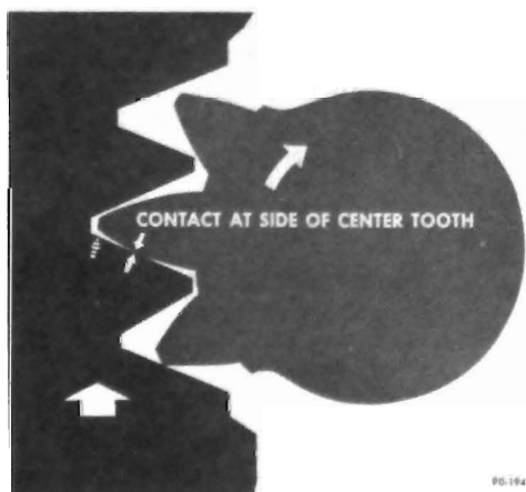
Figure 90-33 - Steering Gear Tooth Contact
