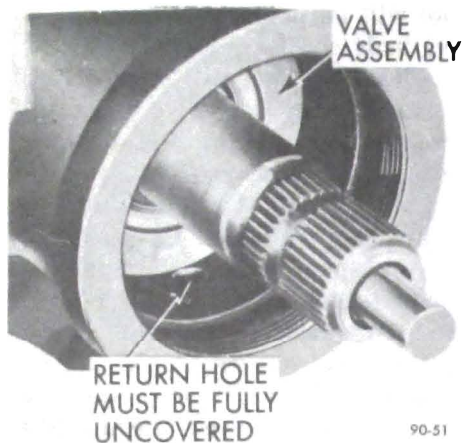
Figure 90-62 Valve Assembly Installed in Housing
