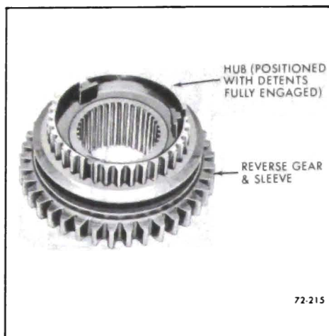
Figure 72-215 - Sliding Sleeve Into Hub
