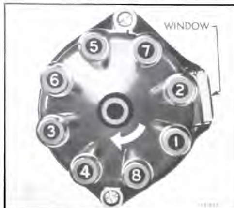
Figure 68-41 - Installing Spark Plug Wires in Cap - V-8 Engines
