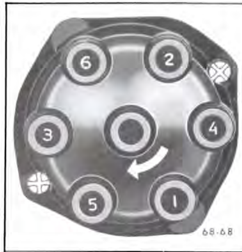
Figure 68-40 - Installing Spark Plug Wires in Cap - L-6 Engine
