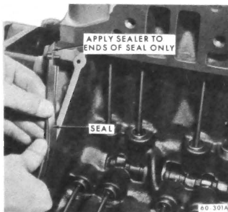
Figure 60-209 Intake Manifold Seal Installation
