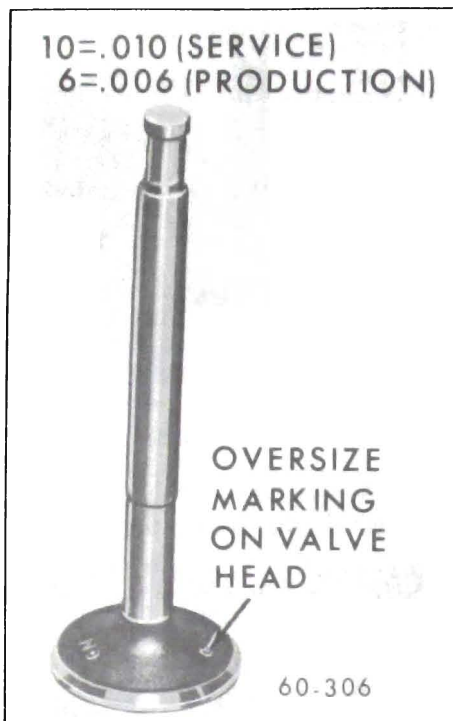
Figure 60-216 Oversize Valve Identification
