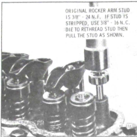
Figure 60-114 - Removing Stripped Rocker Arm Stud
