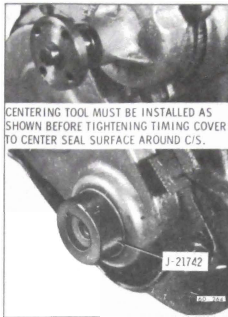
Figure 60-125 - Installing Centering Tool in Cover
