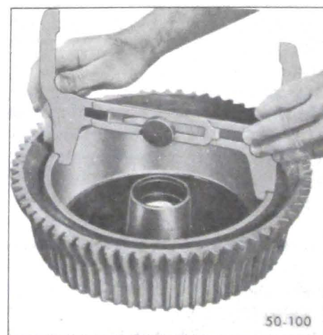
Figure 50-17--Measuring Brake Drum I.D.
