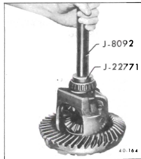
Figure 40-186 - Installing Differential Side Bearing
