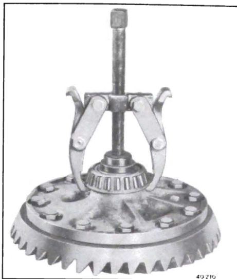
Figure 40-167 Removing Differential Side Bearing
