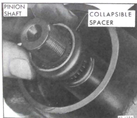
Figure 40-144 Installing Collapsible Spacer
