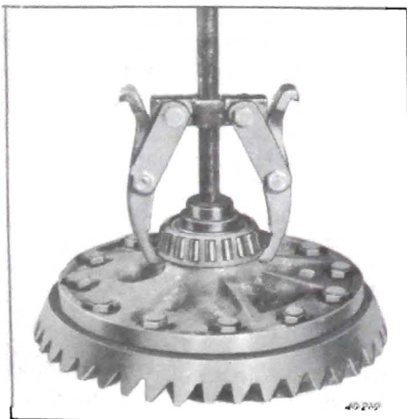
Figure 40-133 Removing Differential Side Bearing
