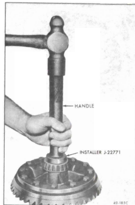
Figure 40-155 Installing Differential Side Bearings
