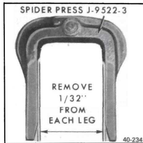
Figure 40-70 - Spider Press Leg Rework
