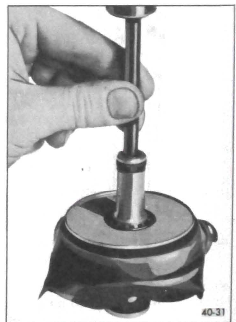
Figure 40-36 - Installing Check Valve
