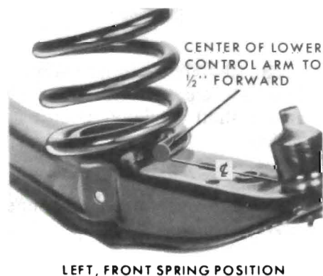
Figure 30-38A - Left Front Coil Spring Position
