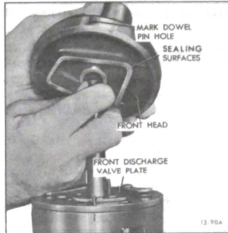
Figure 13-116 Placing Front Head on Cylinder Assembly
