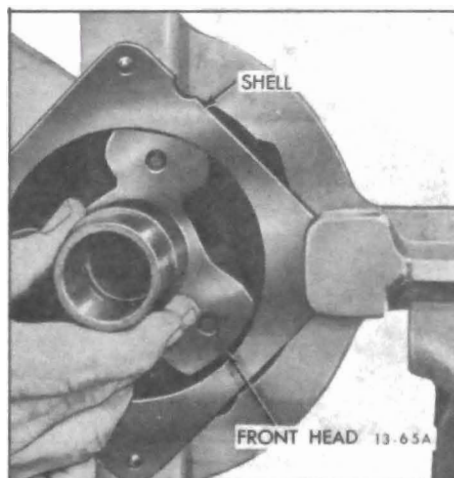
Figure 13-89 Removing Front Head
