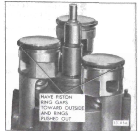
Figure 13-112 Pistons Positioned in "Stair-Step" Arrangement
