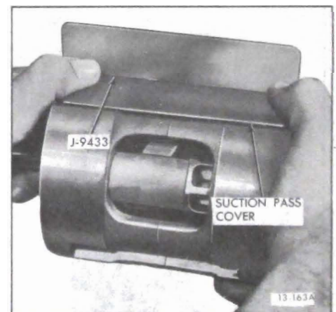
Figure 13-113 Installing Suction Pass Cover
