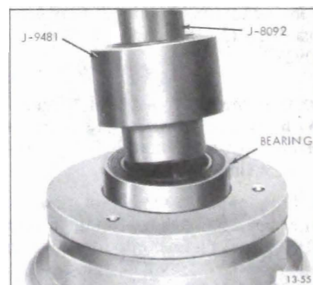
Figure 13-81 Installing Bearing into Pulley Assembly
