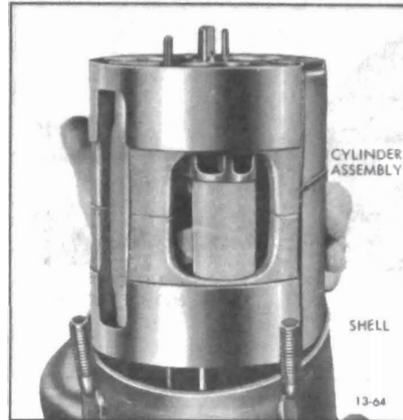
Figure 13-88 Removing Internal Cylinder Assembly
