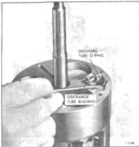
Figure 13-114 Installing Discharge Tube "O" Ring and Bushing
