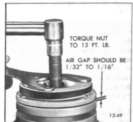
Figure 13-72 Torquing Shaft Nut
