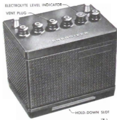
Figure 120-2 Battery - Wildcat, Electra and Riviera
