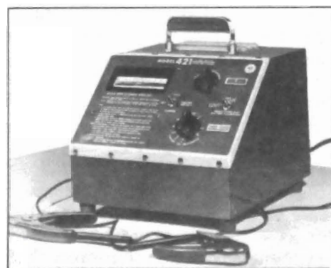
Figure 120-5 421 Battery Tester - Charger
