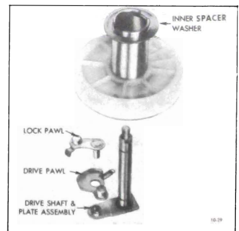
figure 10-46 Disassembling Gear assembly
