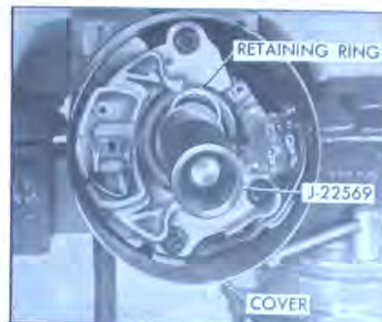
Figure 90-87 Removing Steering Shaft Retaining Ring
