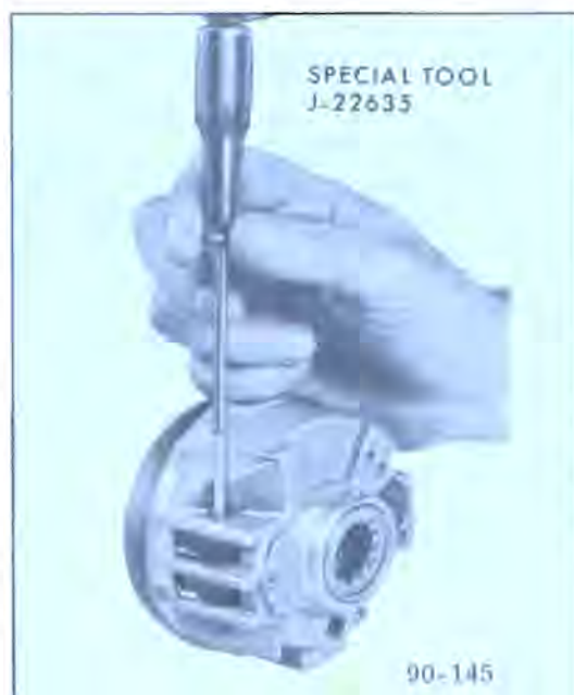
Figure 90-100 Driving Lockshoe Pin Flush With Housing Face
