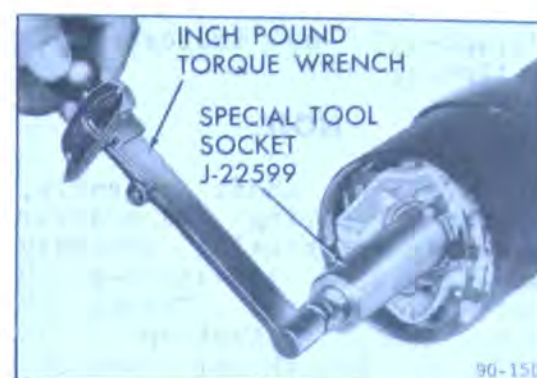
Figure 90-106 Adjusting Steering Shaft Torque
