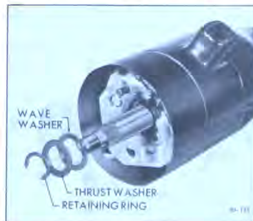
Figure 90-88 Partial Disassembly of Upper Half of Steering Column
