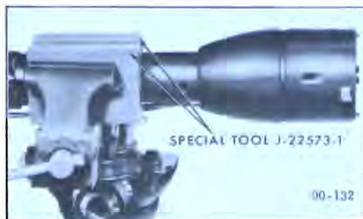
Figure 90-86 Steering Column Installed in Vise
