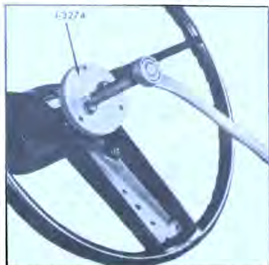
Figure 90-85 Removing Steering Wheel
