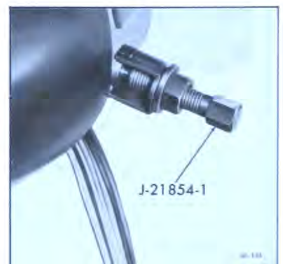
Figure 90-98 Removing Pivot Pins
