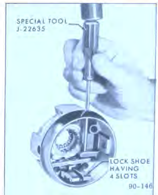
Figure 90-101 Driving Out Release Pin
