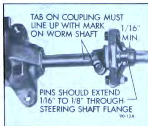
Figure 90-75 Flexible Coupling Installation
