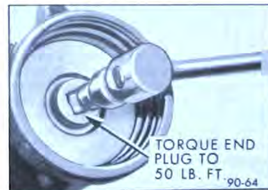
Figure 90-61 Torquing Rack-Piston Nut End Plug
