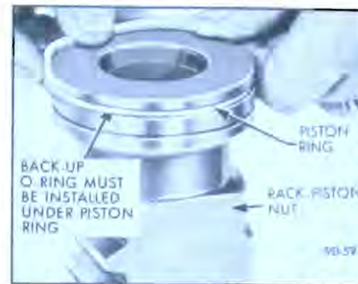
Figure 90-55 Installing Rack-Piston Ring on Rack-Piston Nut
