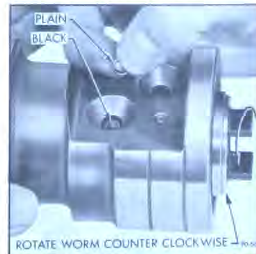
Figure 90-56 Loading Balls in Rack-Piston Nut
