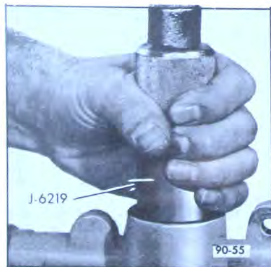
Figure 90-51 Installing Pitman Shaft Seals
