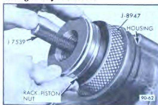
Figure 90-58 Installing Rack-Piston Nut (43-44-45000 Series)
