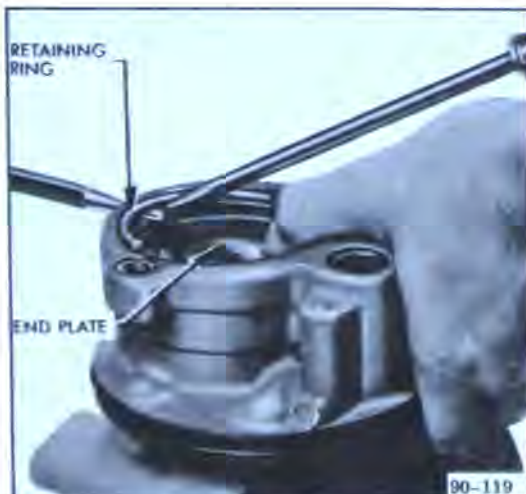
Figure 90-65 Removing End Plate Retaining Ring
