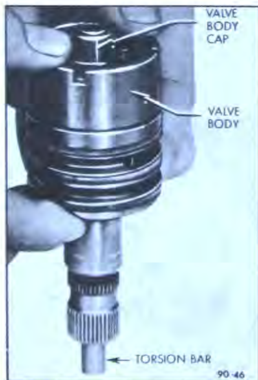
Figure 90-41 Removing Stub Shaft, Torsion Bar and Cap Assembly From Valve Body
