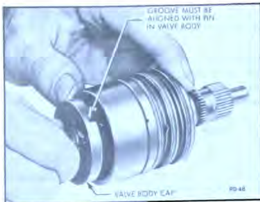
Figure 90-43 Assembling Stub Shaft, Torsion Bar and Cap Assembly in Valve Body
