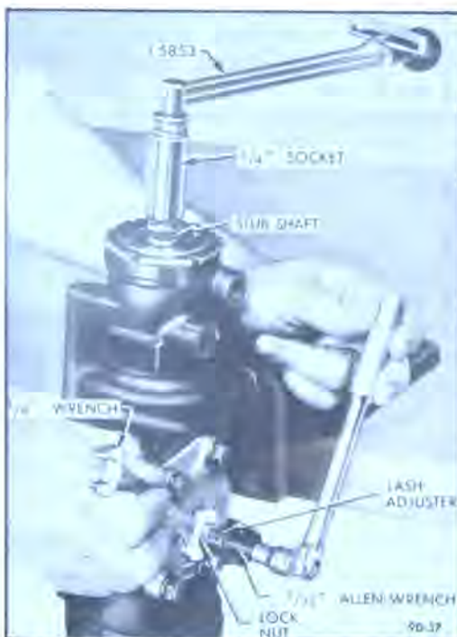
Figure 90-15 Pitman Shaft Overcenter Adjustment
