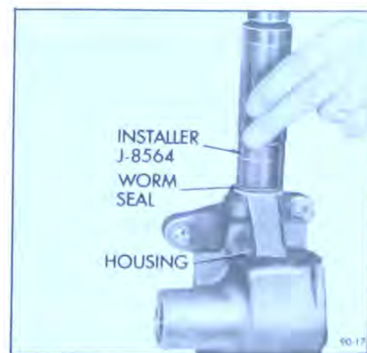
Figure 90-12 Installing Worm Shaft
