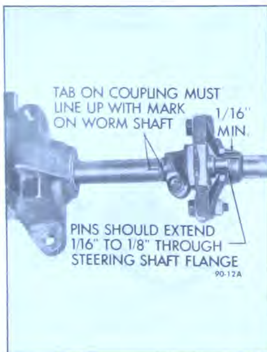
Figure 90-6 Gear Flexible Coupling Installation
