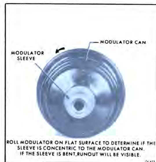
Figure 74-798—Checking Modulator Sleeve Alignment
