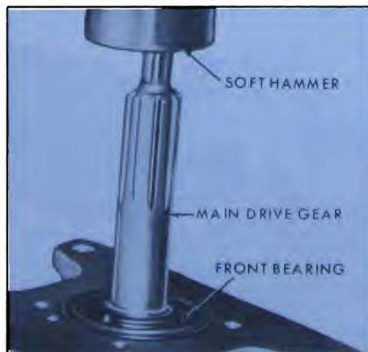
Figure 72-406—Removing Main Drive Gear
