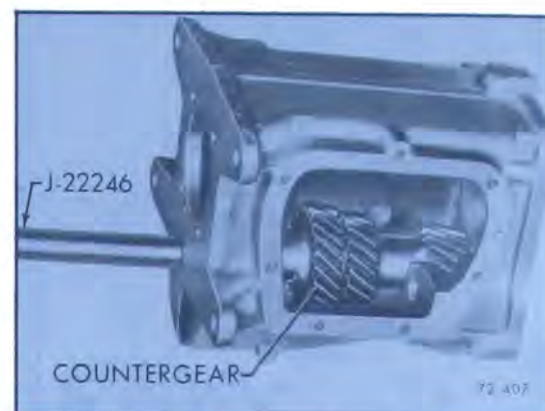
Figure 72-407—Removing Countergear with J-22246
