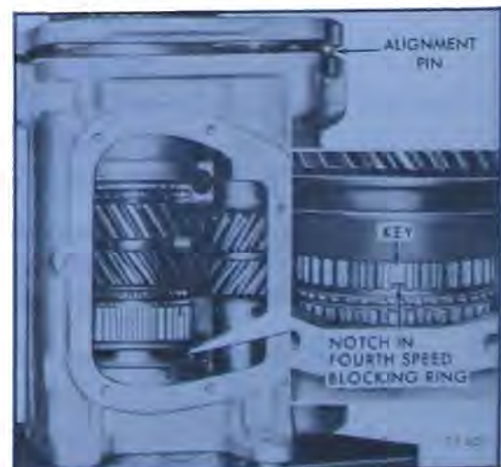
Figure 72-421—Installing Mainshaft Assembly
