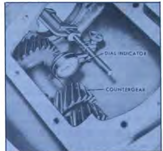
Figure 72-420—Checking Countergear Alignment
