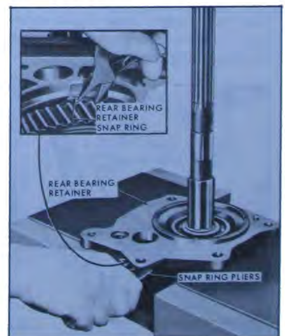
Figure 72-410—Removing Rear Bearing From Retainer
