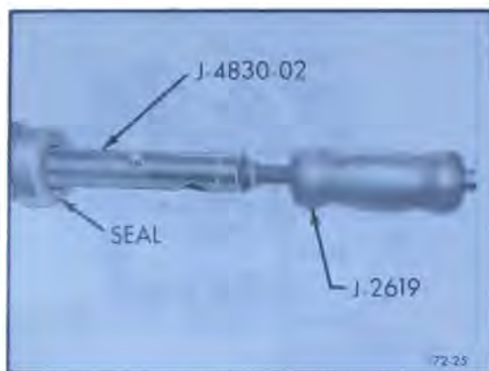
Figure 72-414—Removing Case Extension Oil Seal
