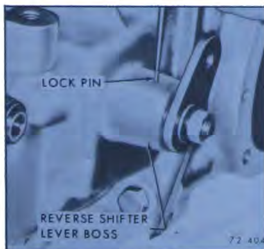
Figure 72-404—Removing Shifter Shaft Lock Pin
