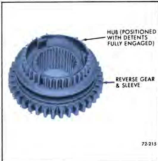
Figure 72-215—Sliding Sleeve into Hub
