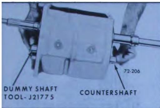
Figure 72-206—Removing Countershaft With J-21775
