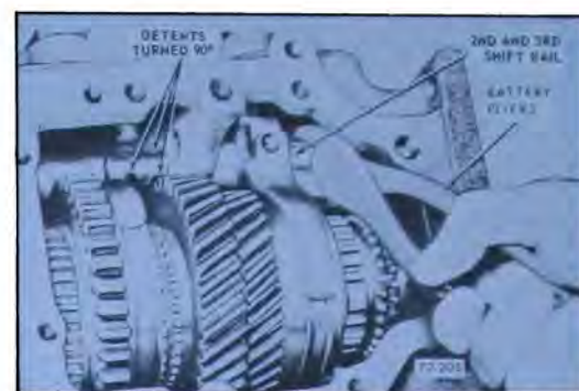
Figure 72-205—Rotating 2nd - 3rd Shift Rail
