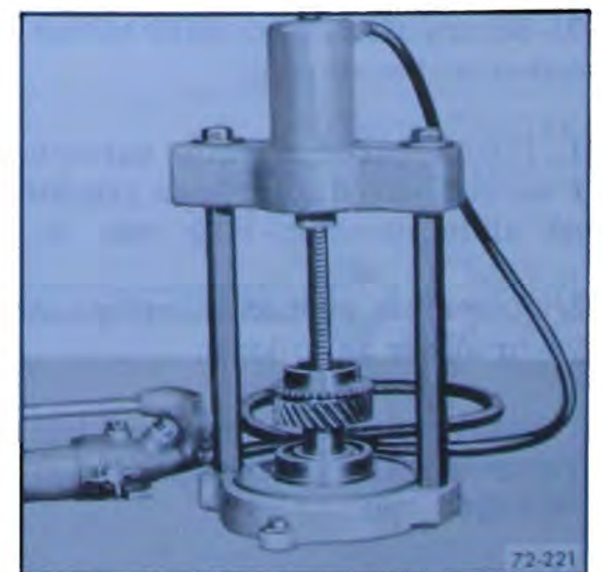
Figure 72-221—Installing Front Main Bearing
