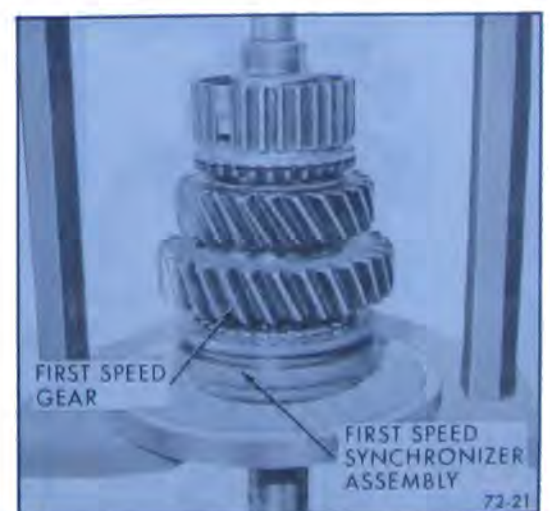
Figure 72-21—Installing First Speed Gear
