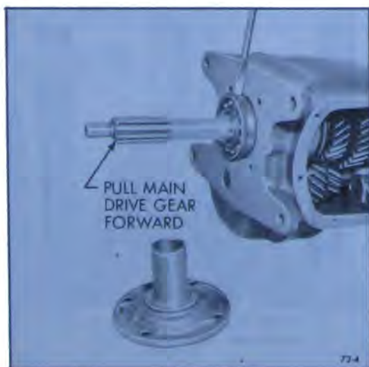
Figure 72-4—Removing Front Main Bearing
