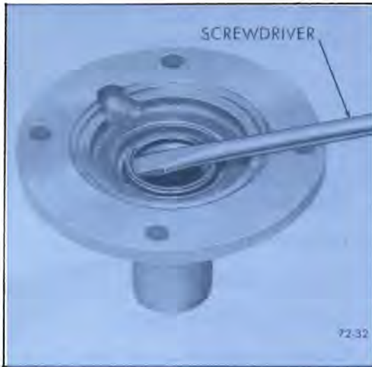
Figure 72-32—Removing Front Bearing Retainer Seal
