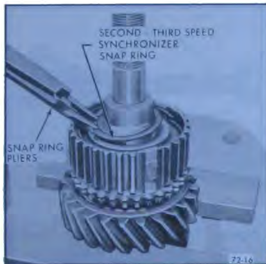
Figure 72-16—Removing Second-Third Speed Synchronizer Snap Ring
