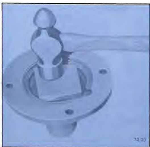
Figure 72-33—Installing Front Bearing Retainer Seal
