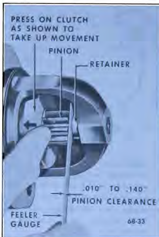
Figure 68-27—Checking Pinion Clearance
