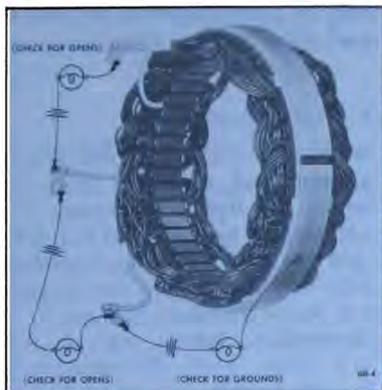
Figure 68-4—Checking Stator for Opens or Grounds
