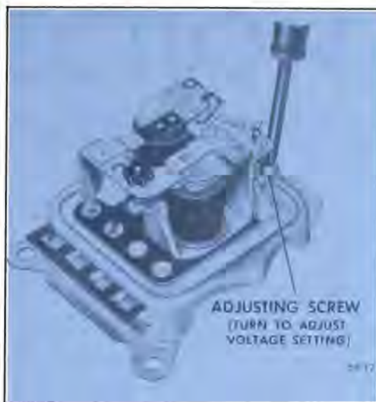
Figure 68-15—Adjusting Voltage Regulator Setting
