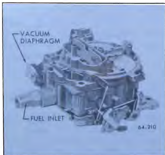
Figure 64-23—Rochester Quadrajets Carburetor
