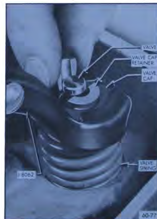
Figure 60-311—Removing Valve Cap Retainers
