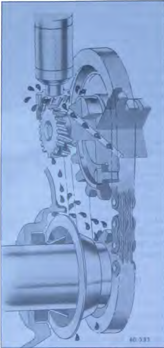
Figure 60-338—Front End Lubrication through a passage to an outlet between the crankshaft sprocket and distributor gear.
