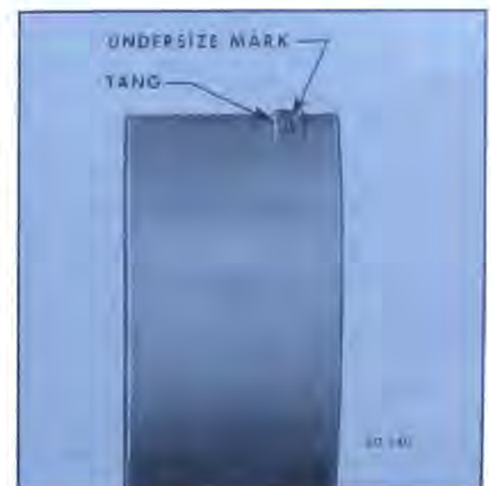
Figure 60-318—Location of Undersize Mark on Bearing Shell
