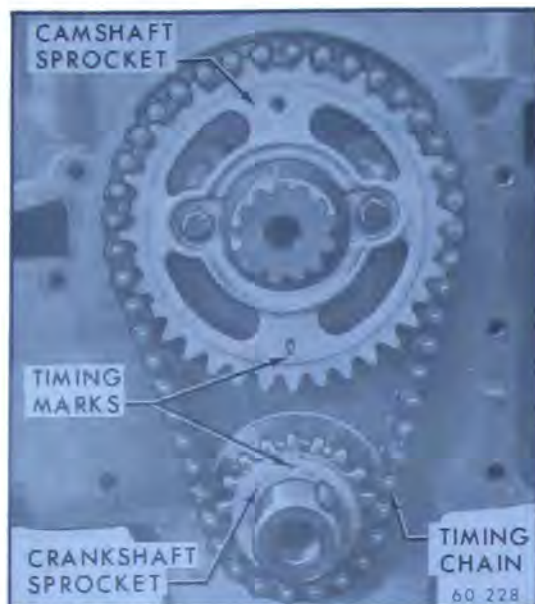
Figure 60-335—Installation of Timing Chain and Sprocket
