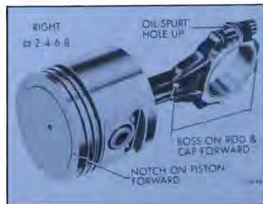
Figure 60-328—Right Bank Piston and Rod Assembly
