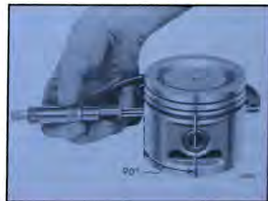
Figure 60-324—Measuring Piston with Micrometer
