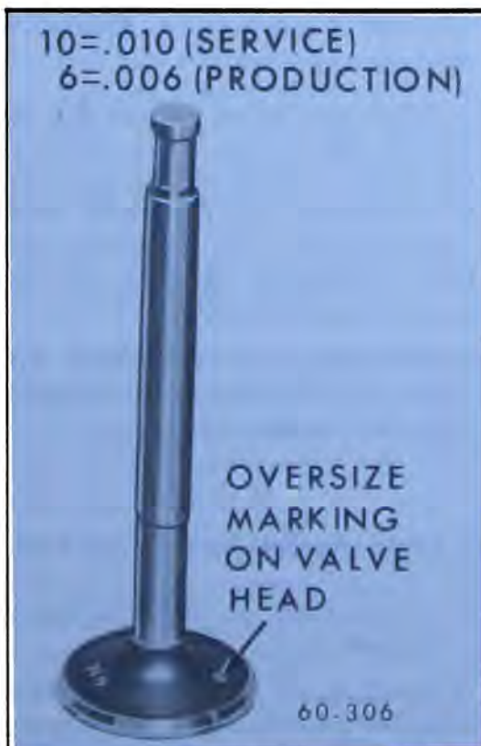
Figure 60-313—Oversize Valve Identification
