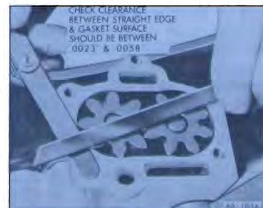
Figure 60-343—Checking Oil Pump End Clearance
