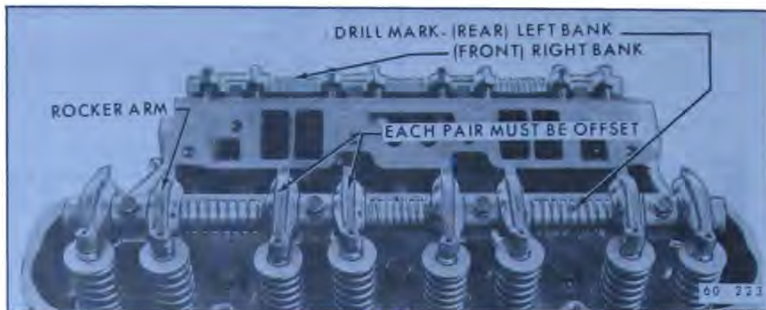
Figure 60-316—Rocker Arm Positioned on Shaft
