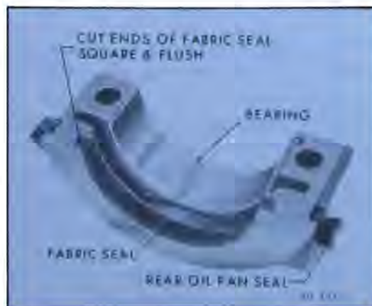
Figure 60-321—Rear Bearing Oil Seal
