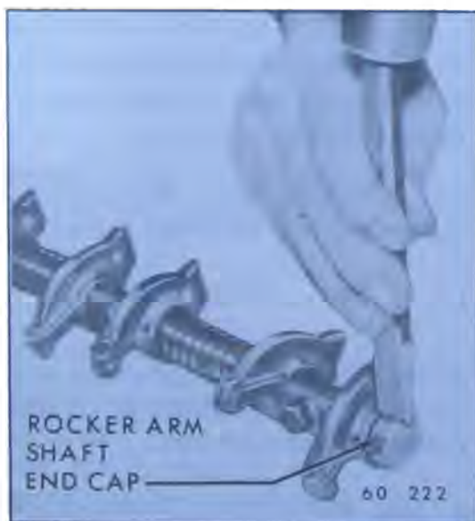
Figure 60-315—Removing Rocker Arm Shaft End Cap
