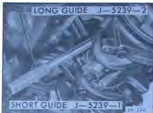
Figure 60-323—Connecting Rod Bolt Guides Installed
