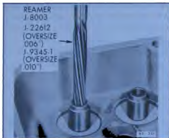
Figure 60-312—Reaming Valve Guide or wire brushes for removing carbon, avoid scratching valve seats and valve faces. A soft wire brush such as J-8358 is suitable for this purpose.
