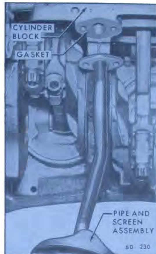
Figure 60-342—Installation of Pipe and Screen Assembly
