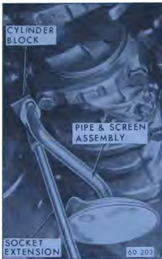
Figure 60-244—Installation of Pipe and Screen Assembly
