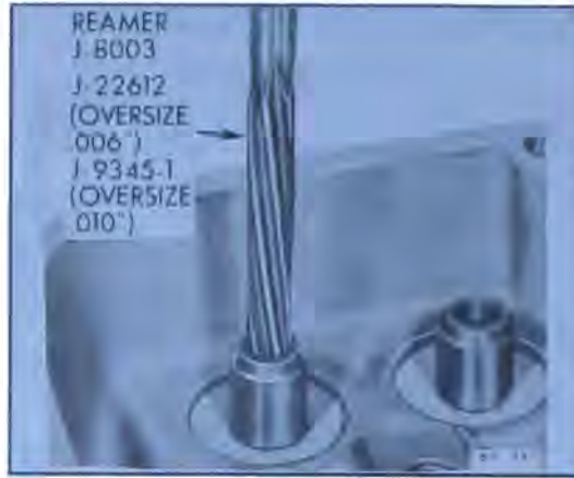
Figure 60-213—Reaming Valve Guide
