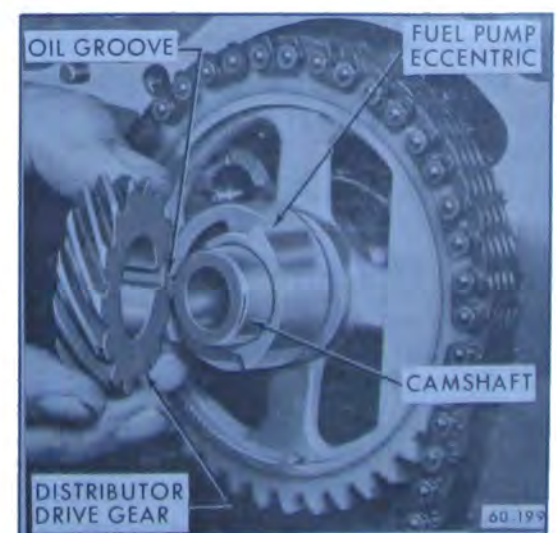
Figure 60-240—Fuel Pump and Distributor Drive Gear Installation
