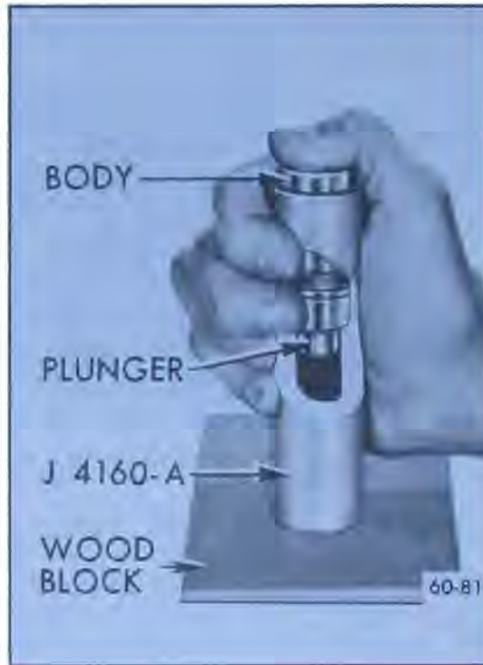
Figure 60-220—Removing Stuck Plunger
