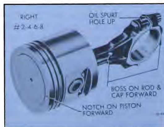
Figure 60-233—Right Bank Piston and Rod Assembly
