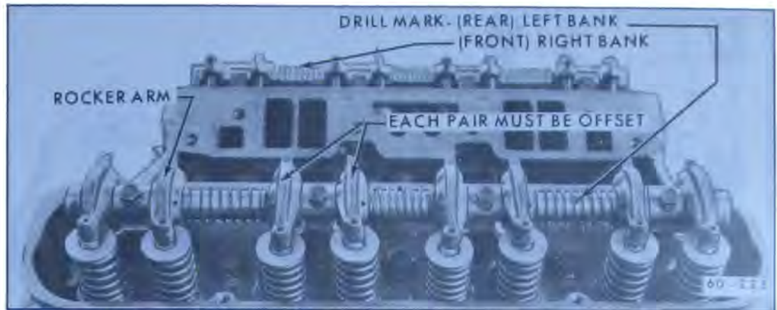
Figure 60-216—Rocker Arm Positioned on Shaft
