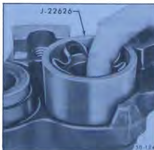
Figure 50-42—Installing Piston Assembly in Bore
