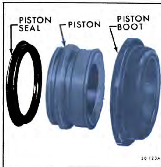
Figure 50-41—Piston - Exploded View
