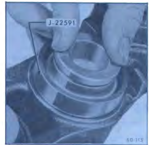
Figure 50-33—Installing Piston Assembly in Bore
