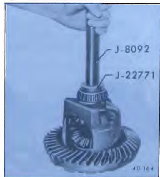
Figure 40-201—Installing Differential Side Bearing
