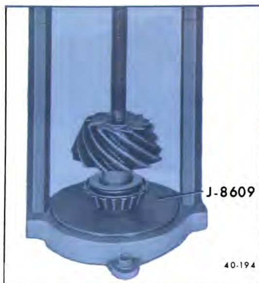
Figure 40-210—Installing Rear Pinion Bearing
