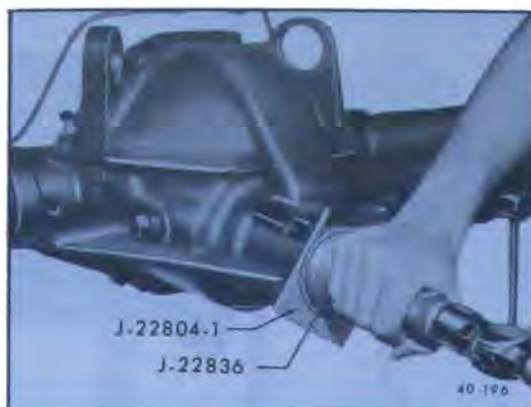
Figure 40-211—Installing Pinion Oil Seal
