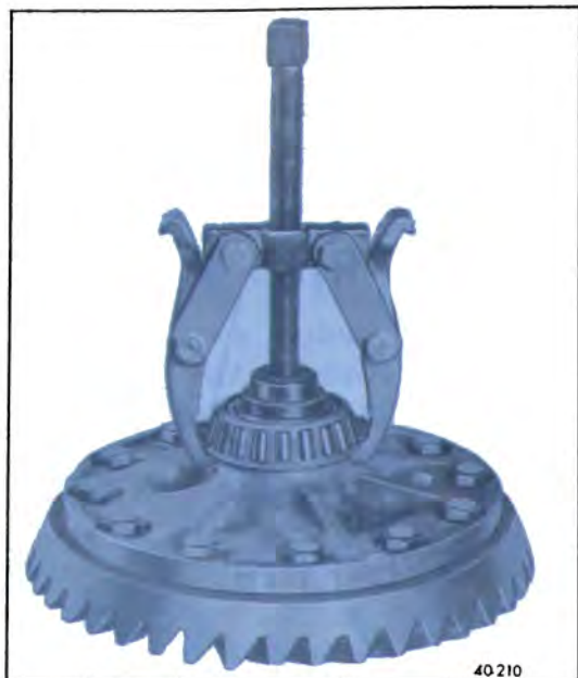
Figure 40-182—Removing Differential Side Bearing
