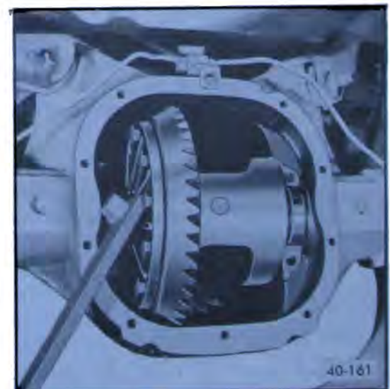
Figure 40-147—Removing Differential Case Assembly
