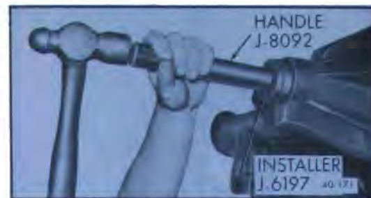
Figure 40-156—Installing Front Pinion Bearing Outer Race
