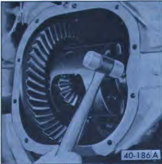
Figure 40-171—Installing Differential Adjusting Shims
