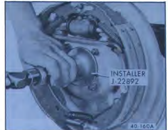
Figure 40-146—Installing Axle Shaft Seal
