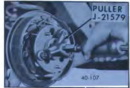
Figure 40-141—Removing Rear Axle Shaft
