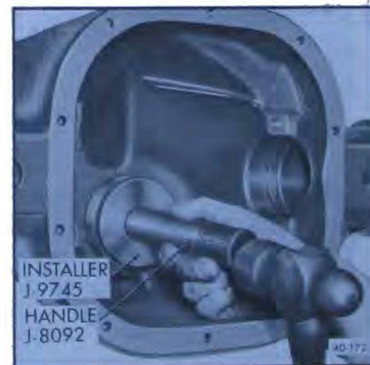
Figure 40-157—Installing Rear Pinion Bearing Outer Race
