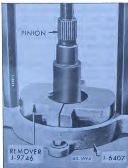
Figure 40-155—Removing Rear Pinion Bearing
