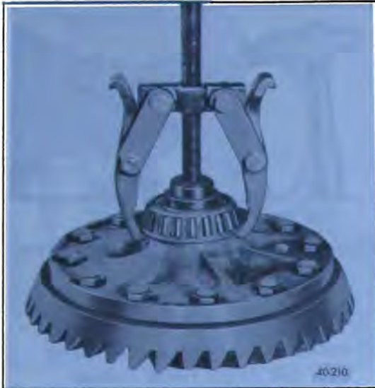
Figure 40-148—Removing Differential Side Bearing
