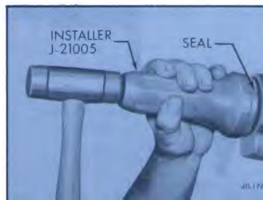
Figure 40-161—Installing Pinion Seal
