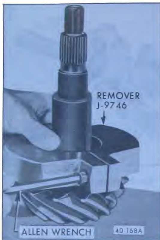
Figure 40-154—Installing Rear Pinion Bearing Remover
