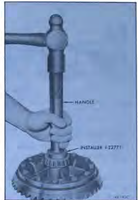
Figure 40-170—Installing Differential Side Bearings
