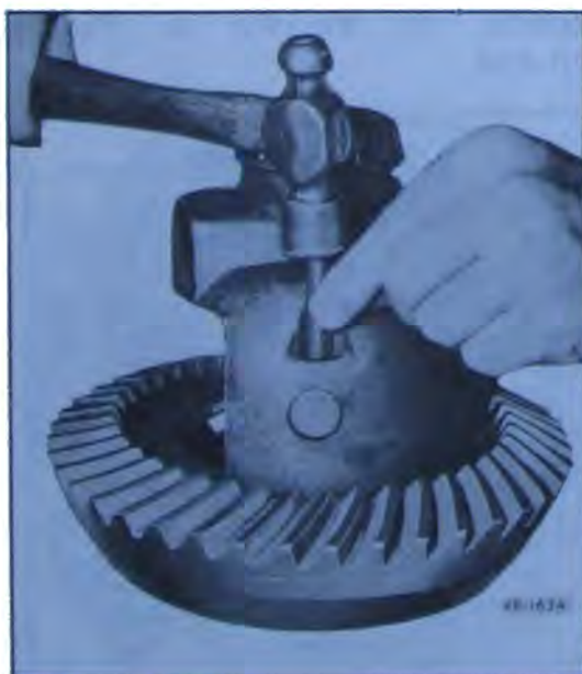
Figure 40-149—Removing Differential Pinion Shaft Pin
