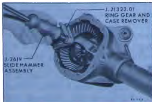
Figure 40-108—Removing Differential Case Assembly
