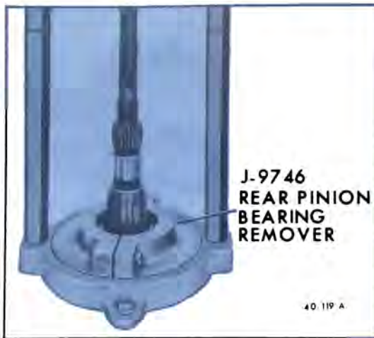
Figure 40-113—Removing Rear Pinion Bearing
