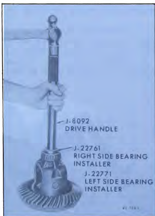
Figure 40-127—Installing Differential Side Bearings
