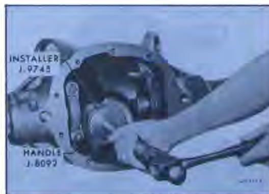
Figure 40-114—Installing Rear Pinion Bearing Outer Race
