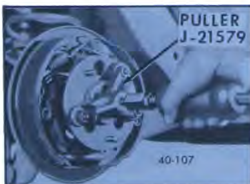
Figure 40-101—Removing Rear Axle Shaft
