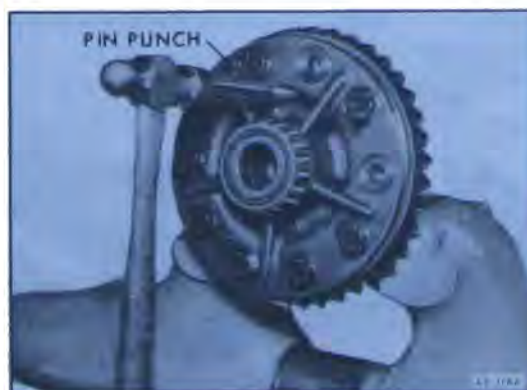
Figure 40-110—Removing Pinion Shaft Roll Pin
