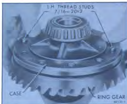
Figure 40-126—Installing Ring Gear on Differential Case
