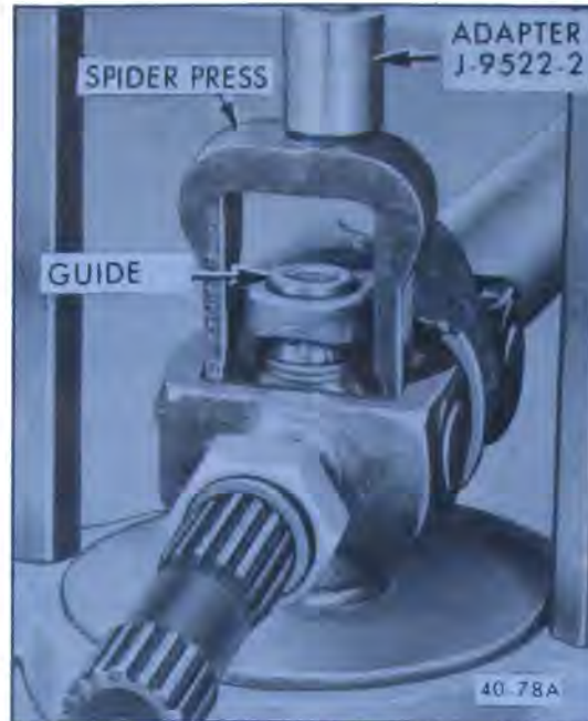
Figure 40-76—Removing Bearing Cap with Guide and Spacer in Place
