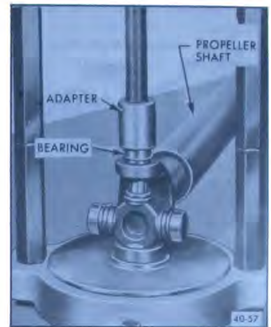
Figure 40-81—Pressing Bearing Cap into Place
