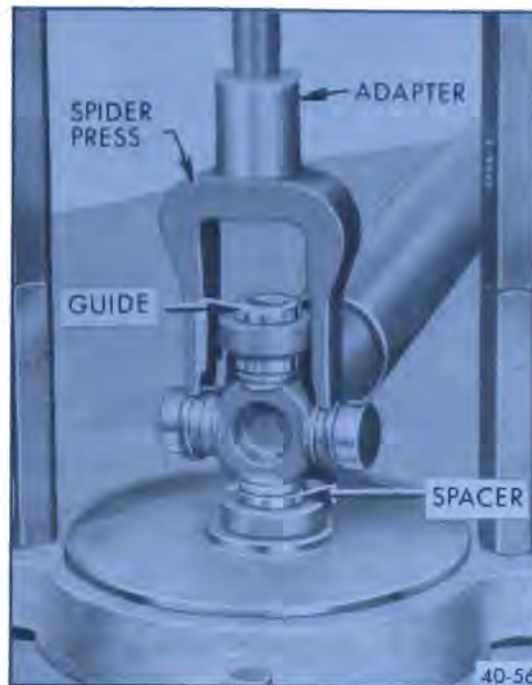
Figure 40-80—Removing Bearing Cap with Guide and Spacer in Place
