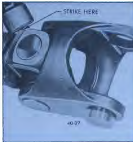
Figure 40-86—Seating U-Joint Snap Rings
