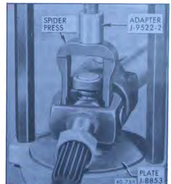
Figure 40-73—Pressing Out Bearing Cap
