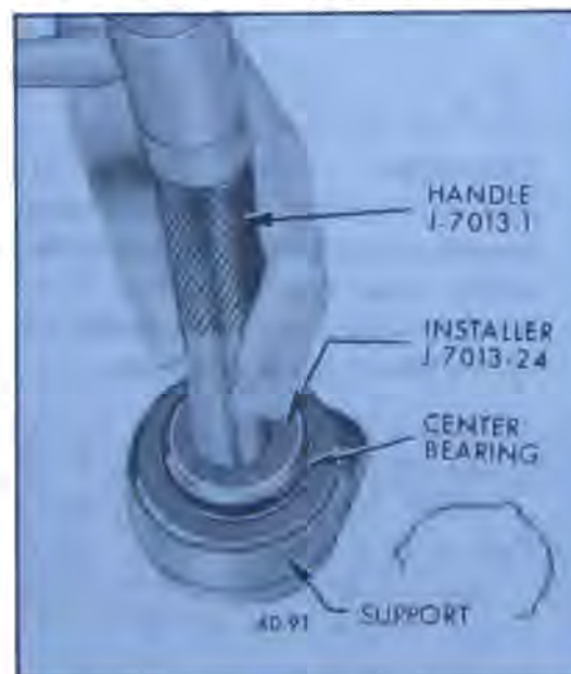
Figure 40-87—Installing Center Bearing into Support
