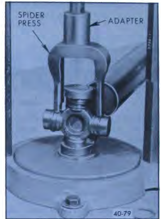
Figure 40-77—Pressing Out U-Joint Bearing Cap
