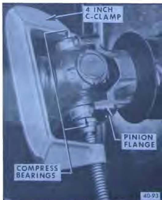
Figure 40-89—Using C-Clamp to Install U-Joint
