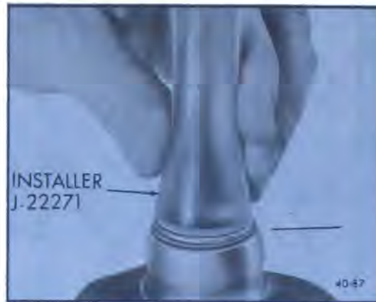
Figure 40-84—Installing Ball Seat Seal
