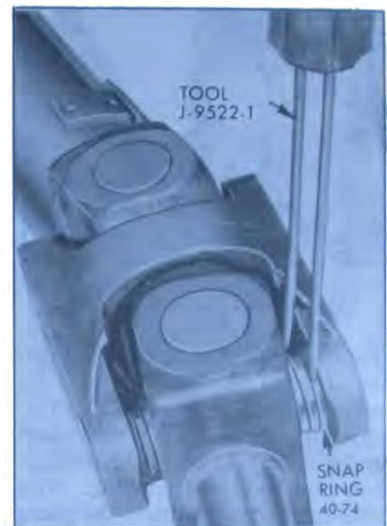
Figure 40-72—Removing Snap Rings from Bearing Cap
