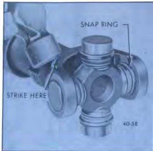
Figure 40-82—Seating U-Joint Snap Rings
